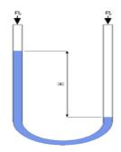
The difference in fluid height in a liquid column manometer is proportional to the pressure difference.
